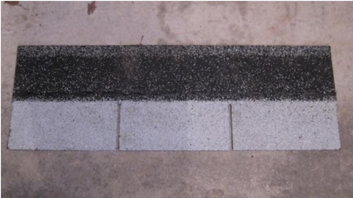
The photo above is a standard three-tab shingle. Each white tab is just under 12-inches wide and the tabs are 5-inches high. The wider black strip above the tabs will be covered by the next row of shingles. If you use these shingles on a roof, all you'll see are the white tabs once all the shingles are installed.
